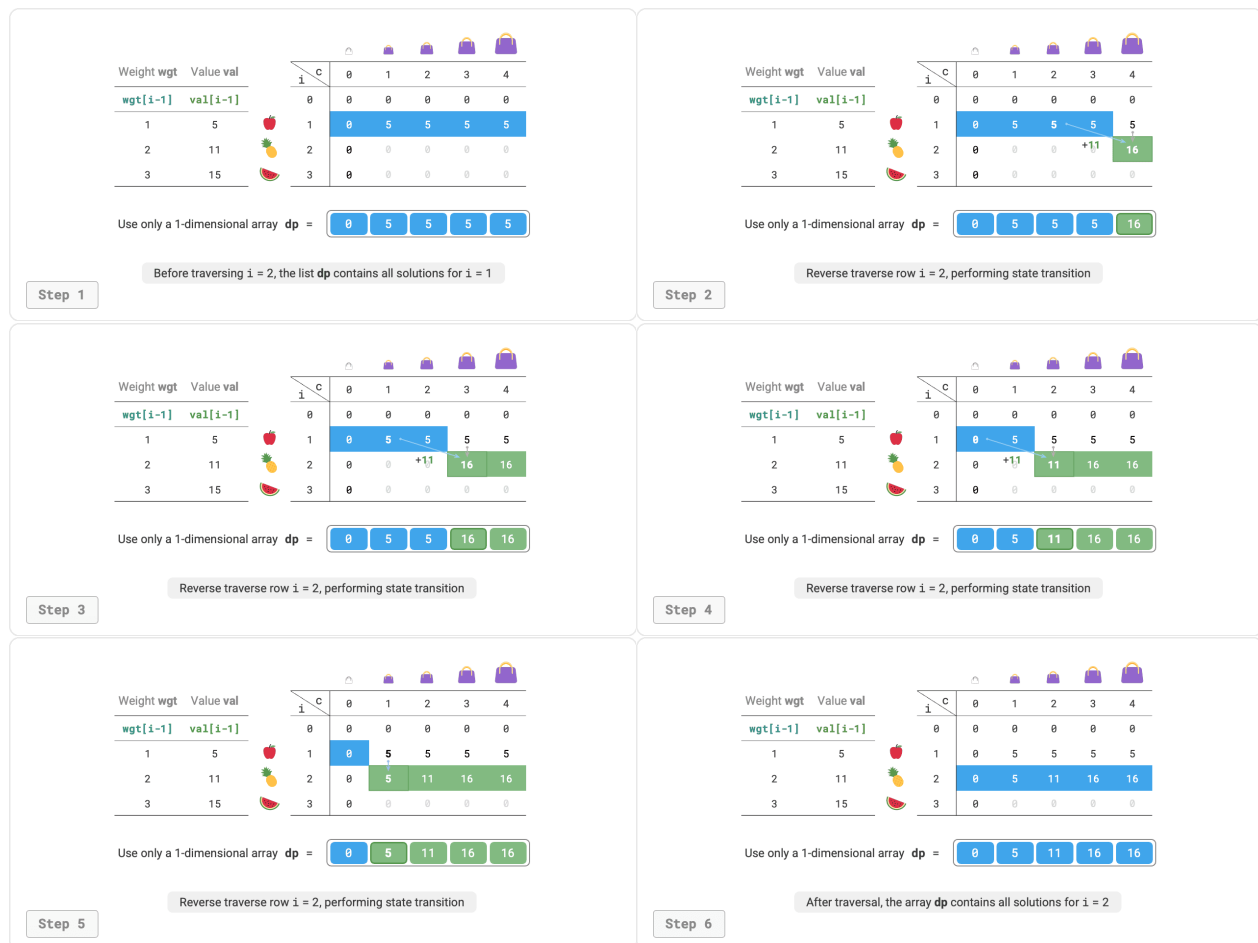
Figure 14-21 Space-optimized dynamic programming process for 0-1 knapsack
