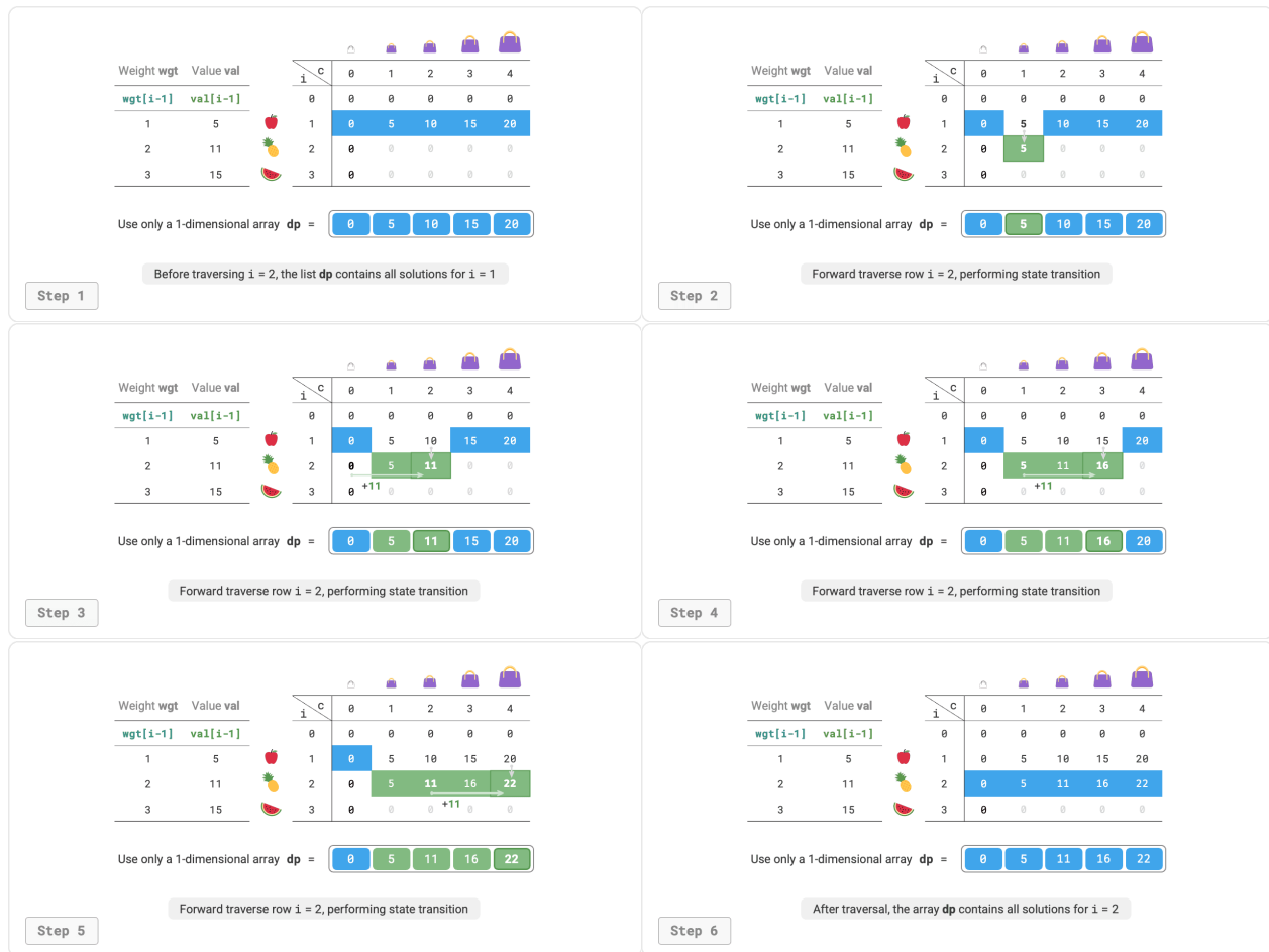
Figure 14-23 Space-optimized dynamic programming process for unbounded knapsack problem
