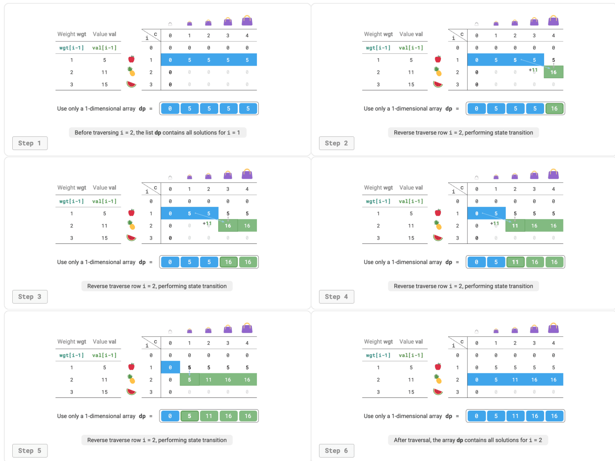
Figure 14-21 Space-optimized dynamic programming process for 0-1 knapsack
