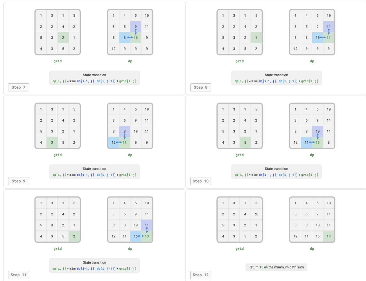
Figure 14-16 Dynamic programming process for minimum path sum
