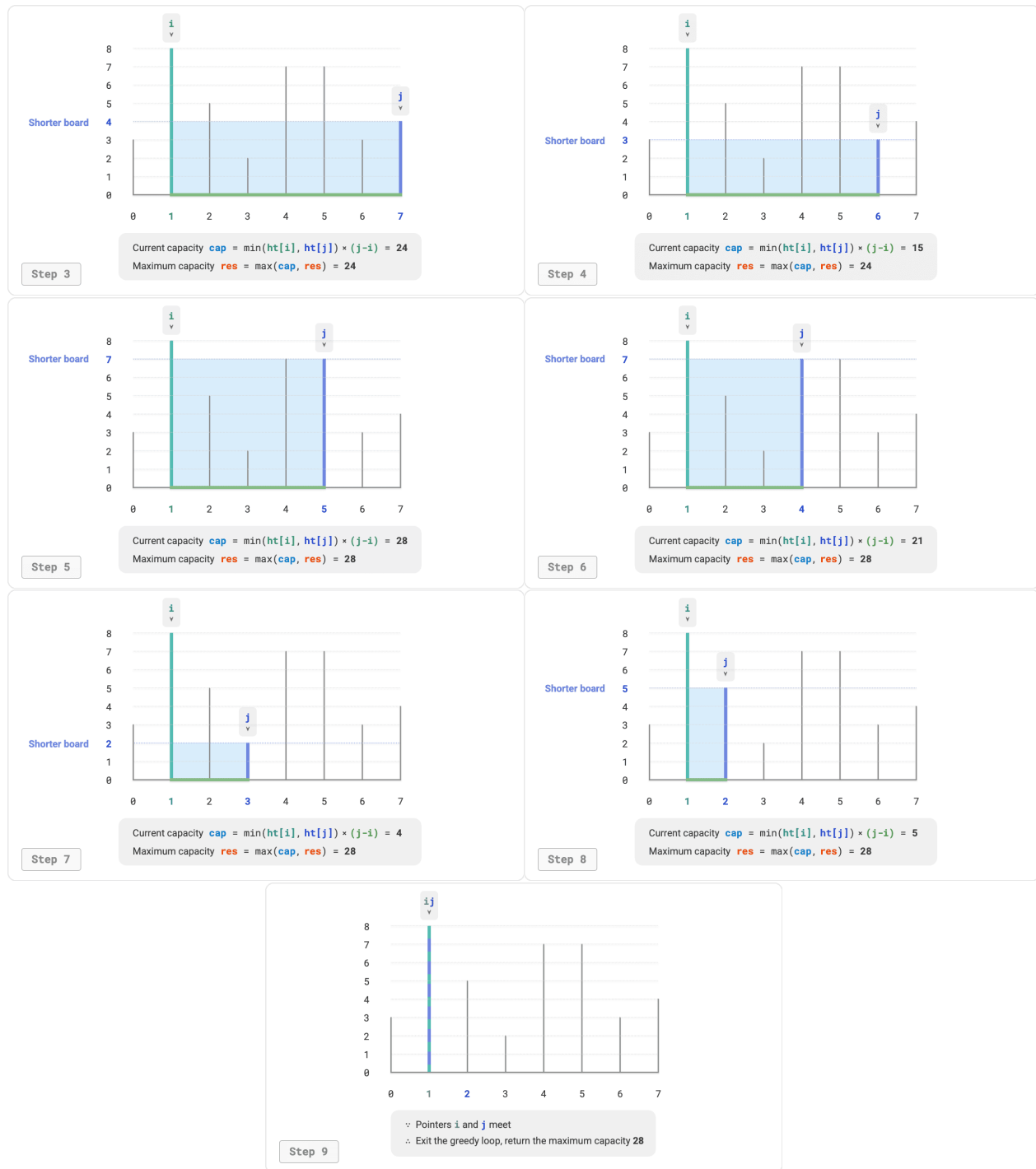
Figure 15-11 Greedy process for the max capacity problem
